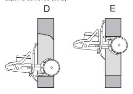
The blade guards are designed to easily adapt to how deep in the work piece the power cutter is moved.
